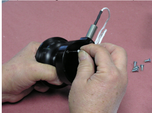
Figure 7 Installation of MTH Alignment Pin
