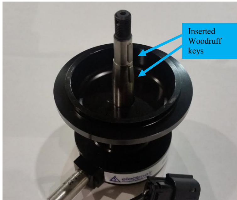
Figure 24: Impulse Coupled MTH Shaft with Woodruff Keys inserted. Step 4b
