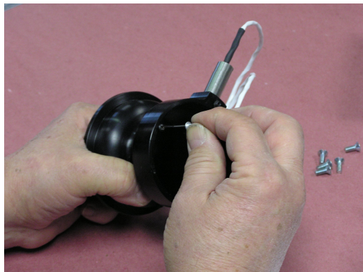
Figure 23: Installation of MTH Alignment Pin on an EA-3000 MTH
