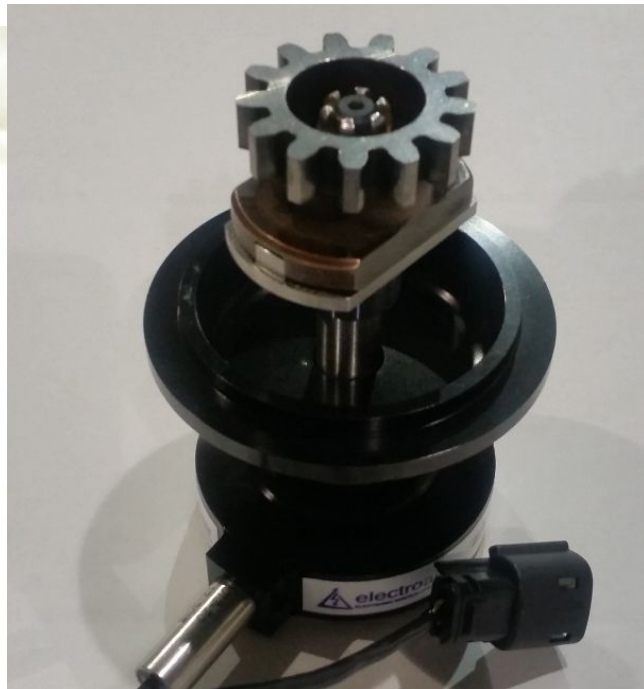
Figure 26: Drive Gear installed on MTH. Step 4d
