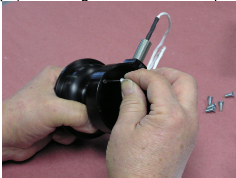
Figure 2: Installation of MTH Alignment Pin
