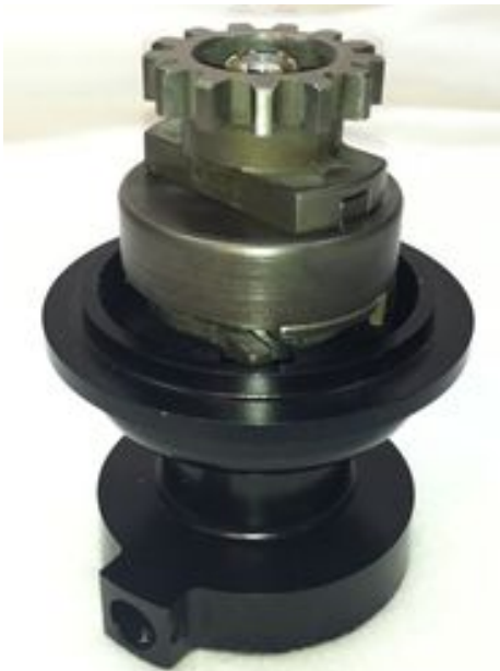
Figure 5: Drive Gear installed on MTH. Step 4d
