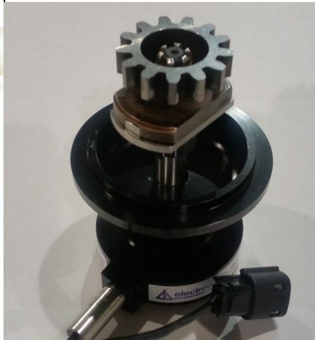
Figure 5: Drive Gear installed on MTH. Step 4d
