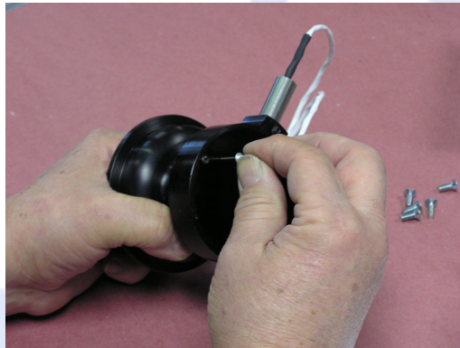
Figure 2: Installation of MTH Alignment Pin
