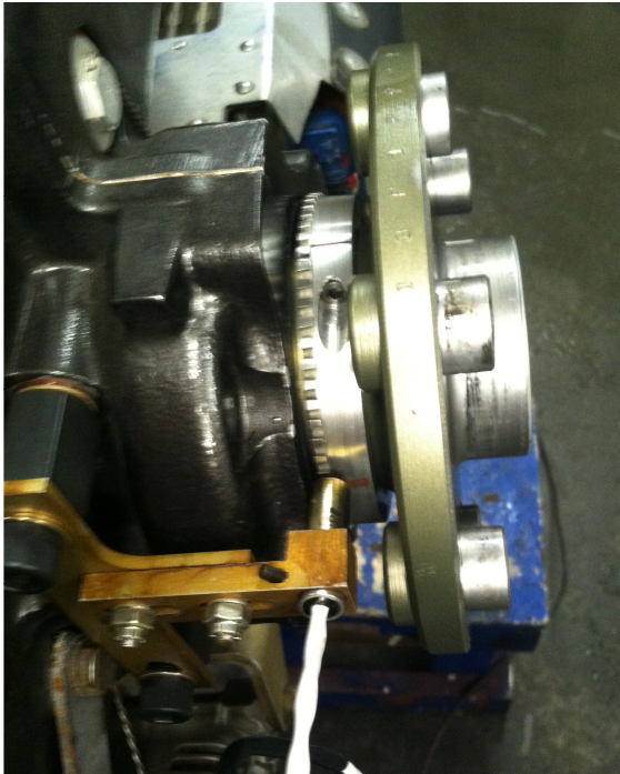
Figure 9: Picture of components that make up the Lycoming CSTW Sensor Bracket; 1. Pick-Up Bracket; 2. Pick-Up Holder; 3. Magnetic Pick-up (Magnetic Sensor); hardware is not shown for clarity.
