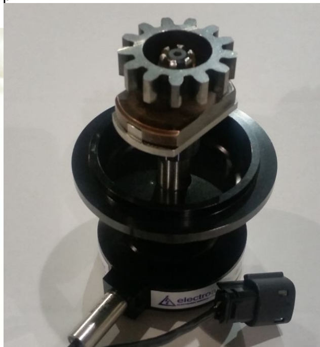
Figure 5: Drive Gear installed on MTH. Step 4d
