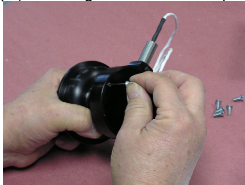
Figure 2: Installation of MTH Alignment Pin
