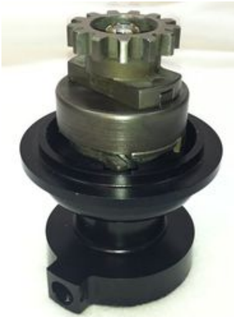
Figure 26: Drive Gear installed on MTH. Step 4d
