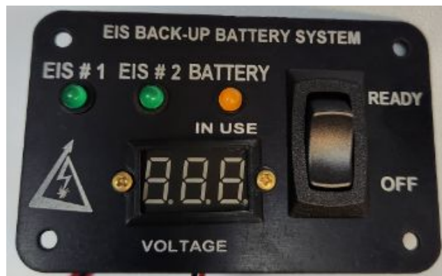
Figure 1: EIS Back-up Battery System Panel
