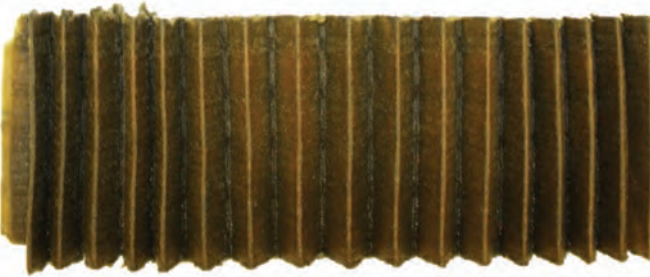
Inspect the filter pleats for metal particles and other materials.
