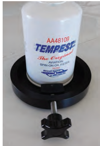
Oil filter cutting tools remove the case without introducing metal into the filter.
