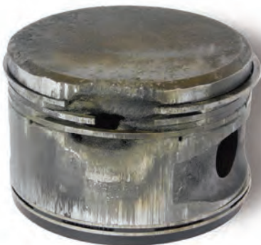
FIGURE 1 Piston destroyed by excessive pre-ignition detonation.
