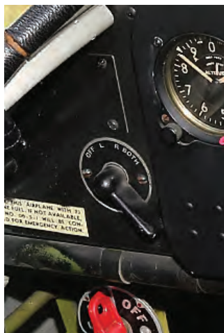
Original Stearman Dixie magneto switch
