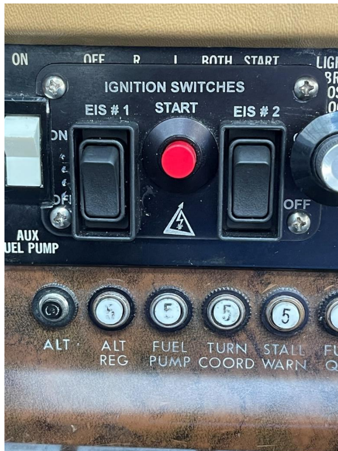
EIS Switch Panel, notched to fit the Cessna Key hole area
