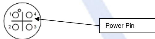
Figure 5: Coil Pack Connector typically located on the engine side of the firewall plugged into the coil pack. Measure from pin 4 for voltage reading.
