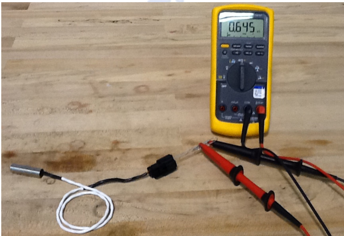
Figure 1: Measurement of Mag Sensor Resistance. Measure from red wire to black wire.
