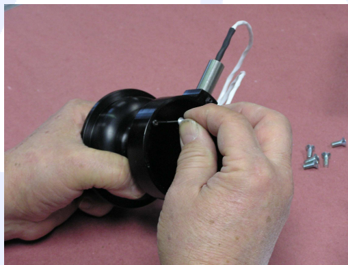
Figure 3.1: Installation of MTH Alignment Pin
