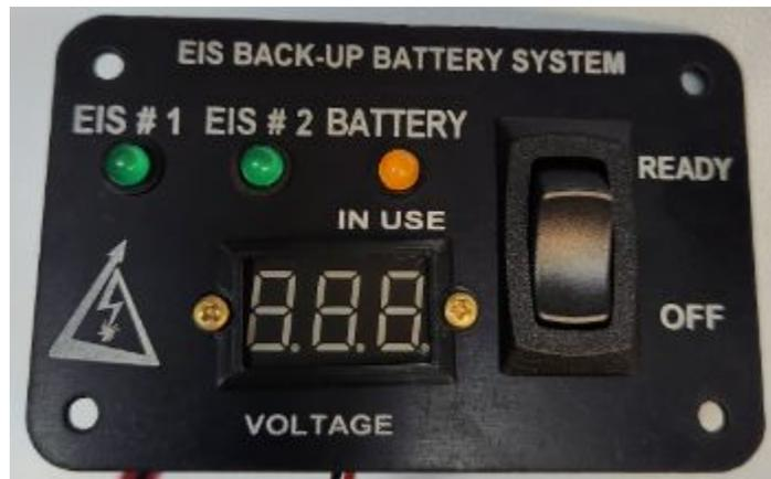
Figure 1: EIS Back-up Battery System Panel
