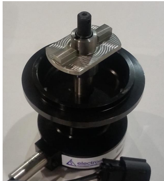
Figure 4: Impulse Coupler and Faux Impulse Coupler Installed. Step 4c
