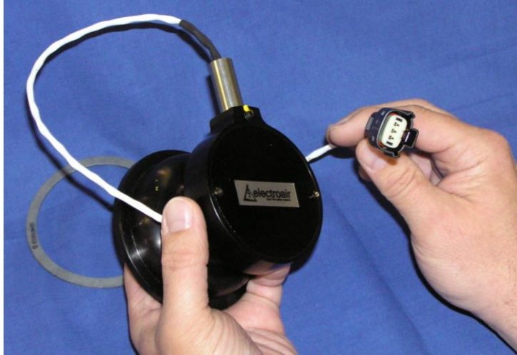
Figure 17: MTH and 3 Pin Female Connector
