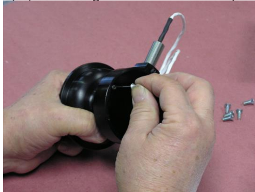
Figure 28: Installation of MTH Alignment Pin
