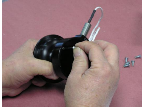
Figure 2: Installation of MTH Alignment Pin
