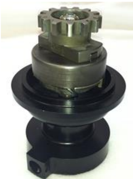
Figure 5: Drive Gear installed on MTH. Step 4d
