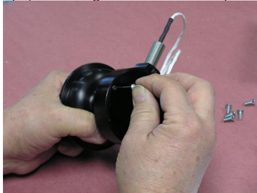
Figure 7 Installation of MTH Alignment Pin
