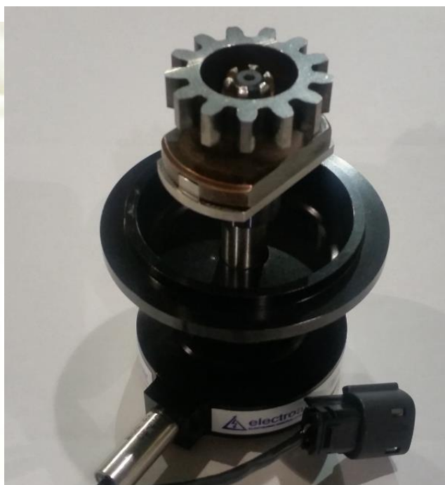
Figure 26: Drive Gear installed on MTH. Step 4d
