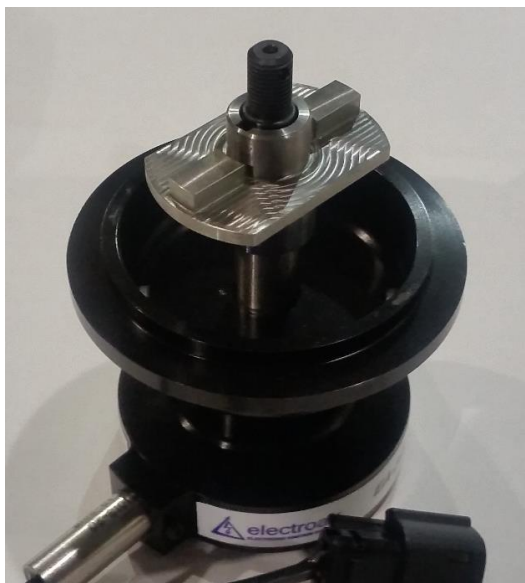
Figure 25: Impulse Coupler and Faux Impulse Coupler Installed. Step 4c
