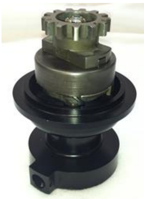
Figure 26: Drive Gear installed on MTH. Step 4d
