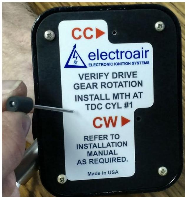
Figure 7: Installation of MTH Alignment Pin
