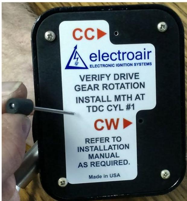
Figure 7: Installation of MTH Alignment Pin
