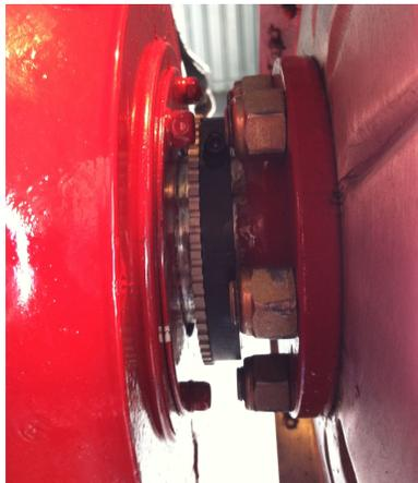
**Figure 2: Typical installation of CSTW on a Continental 470 engine. Note: Minimum clearance of 0.650 inches required between front of case and rear of prop studs; contact Electroair Tech Support for additional information.**
