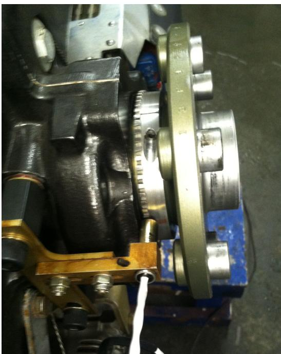
**Figure 4: Typical installation of CSTW on a Lycoming 540 engine. Picture shows orientation of trigger wheel and typical bracket location. Please contact Electroair Tech Support if there are any questions about the assembly.**
