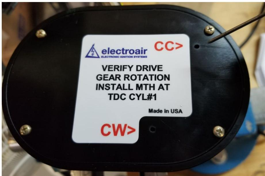
**Figure 10: Installation of MTH Alignment Pin**
