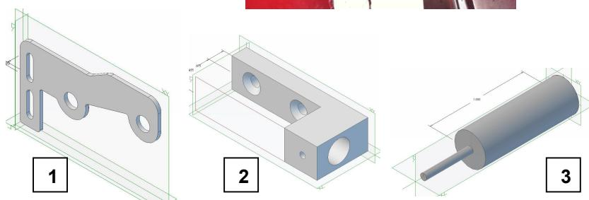
**Figure 3: Components that make up the Continental CSTW Sensor Bracket;** 1. Pick-Up Bracket (rear-mount alternator; front-mount alternator bracket not shown); 2. Pick-Up Holder; 3. Magnetic Pick-up (Magnetic Sensor)
