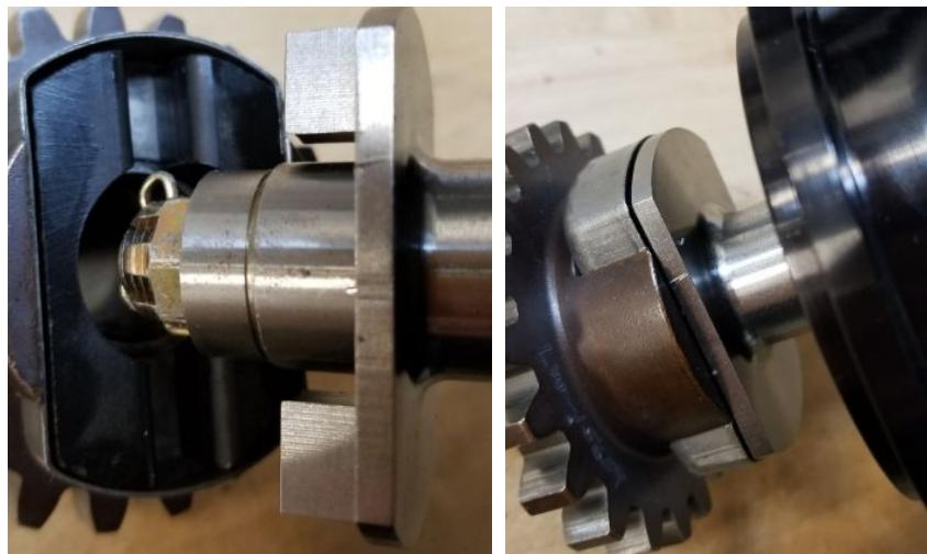
**Figure 11: MTH Installation into magneto drive gear/cushions**
