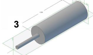
**Figure 5: Components that make up the Lycoming CSTW Sensor Bracket; 1. Pick-Up Bracket; 2. Pick-Up Holder; 3. Magnetic Pick-up (Magnetic Sensor); hardware is not shown for clarity.**
