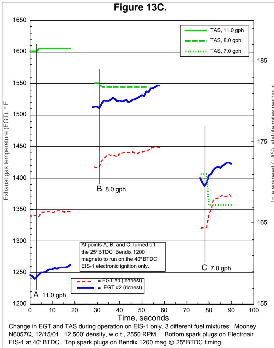
again reflecting the amount of energy wasted by fuel burning after it exits the exhaust valve. But two effects are occurring simultaneously. One is the influence of firing only the top spark plug in each cylinder. The other is the effect of retarding the timing from 40° BTDC to 25° BTDC.
