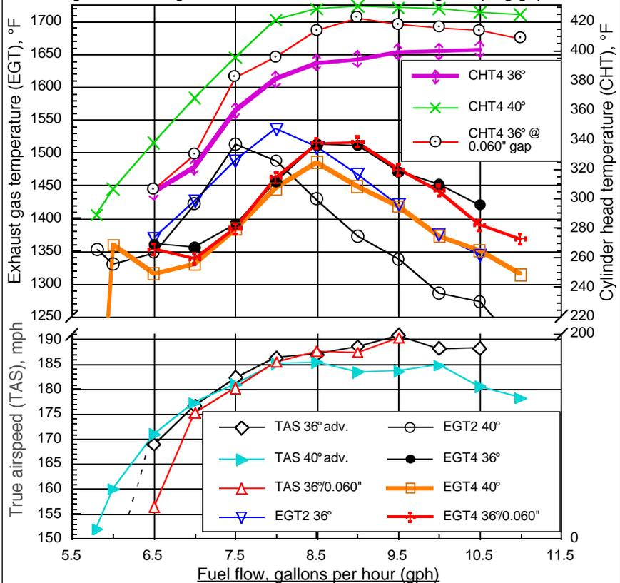
Mooney N6057Q: IO-360A1B6X engine. 12,500' density altitude. Electroair EIS-1 firing bottom plugs using 0.031" gap, Bendix 1200 magneto @ 25° BTDC firing top plugs using 0.018" gap. Wide open throttle, 2550 RPM, All CHT's corr. to 100° F day. Cyl # 4 (leanest) bottom plug gap = 0.060" on 1/10/02 flight only. Aircraft weights: 2472 lb. @ 36°, 2537 lb. @ 40°, 2490 lb. @ 0.060" gap.
