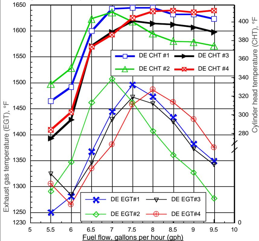
Mooney N6057Q; 15,000' density alt., wide open throttle, 2550 RPM, Vetter DAD records. CHT corrected to 100 °F day. DE = dual electronic EIS-1 ignitions @ 41° BTDC timing. Note cylinder #2 clearly has the richest mixture at any fuel flow.
