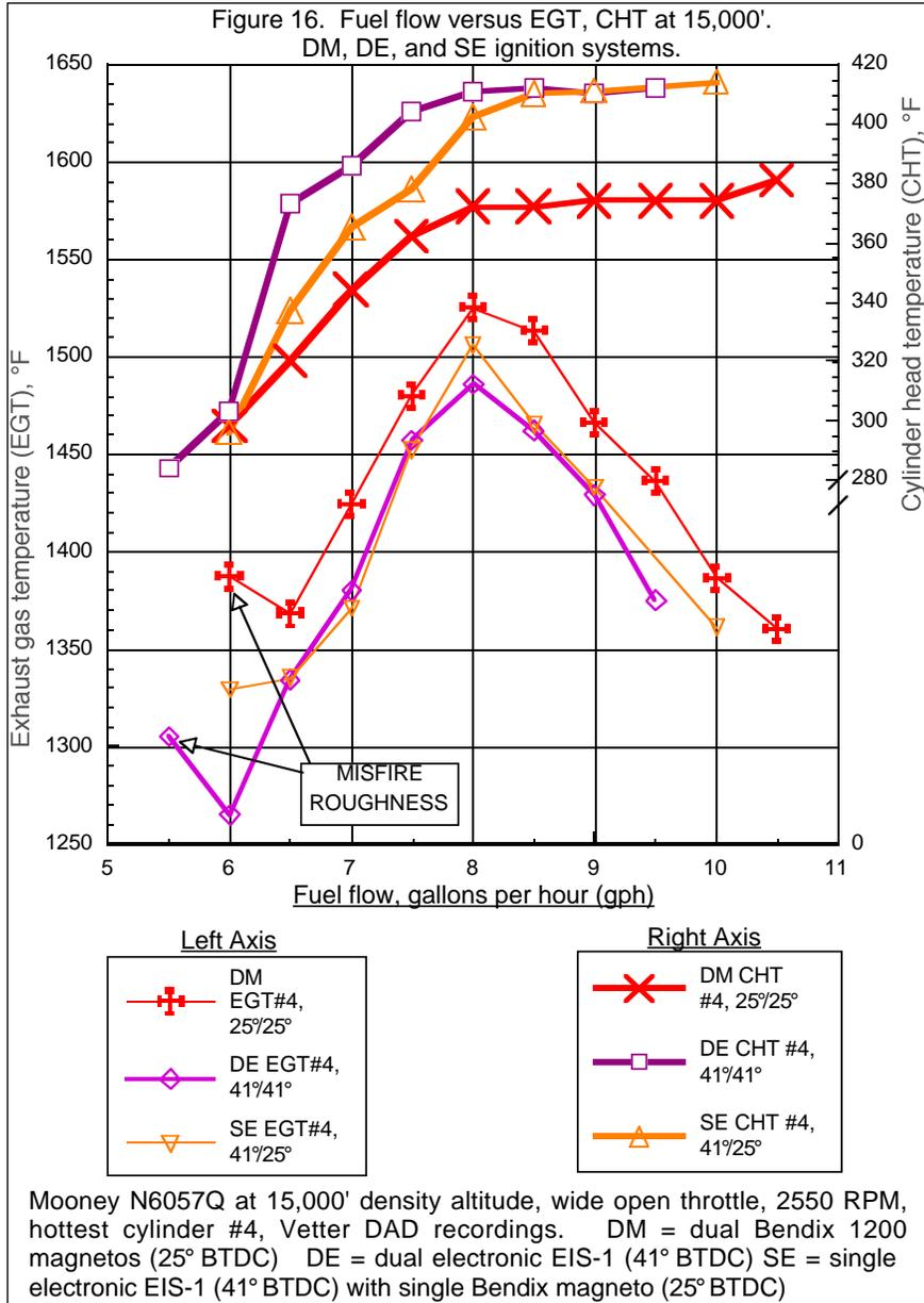
Mooney N6057Q at 15,000' density altitude, wide open throttle, 2550 RPM, hottest cylinder #4, Vetter DAD recordings. DM = dual Bendix 1200 magnetos (25° BTDC) DE = dual electronic EIS-1 (41° BTDC) SE = single electronic EIS-1 (41° BTDC) with single Bendix magneto (25° BTDC)
