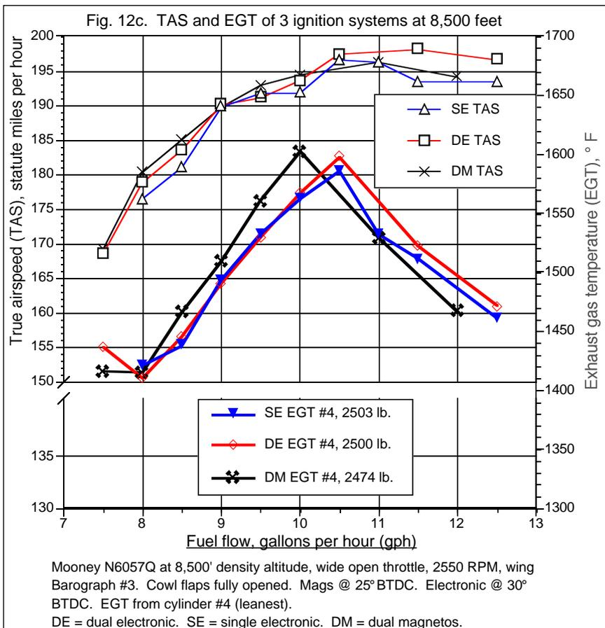
acceptable for continuous operation. At 7.0 gph, where no misfiring was evident, the DM system shows a TAS of 167.8 mph, 5.6 mph slower than DE system, while using 7.7% more fuel. These figures apply to operation at about 130-200° F lean of peak EGT, i.e., very lean.
