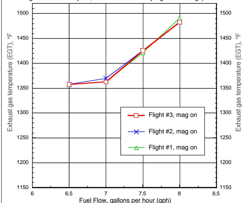
Mooney N6057Q at 12,500' density altitude. SE config., wide open throttle, 2550 RPM, Vetter DAD recordings. EIS-1 fires bottom plugs at 36° BTDC with 0.031" gap. Bendix Magneto @ 25° BTDC fires top plugs with 0.018" gap. Cylinder #2 (richest) has its plug electrode axes remaining at stock rotation on all 3 flights while cylinder #4 has its bottom plug gap rotations set to #1 = -30°, #2 = +60°, #3 = +10°. Figure 20a shows gap rotation effects on EGT.
