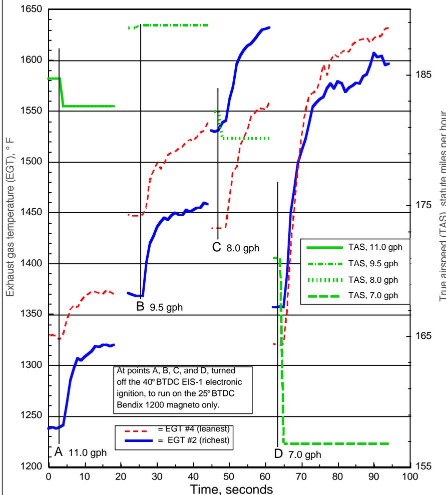
Change in EGT and TAS during operation on left magneto only, 4 different fuel mixtures: Mooney N6057Q, 12/15/01. 12,500' density, w.o.t., 2550 RPM. Bottom spark plugs on Electroair EIS-1 at 40° BTDC. Top spark plugs on Bendix 1200 mag @ 25° BTDC timing.
