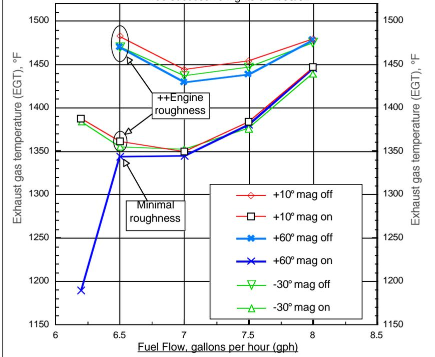
Mooney N6057Q; SE ignition at 12,500' wide open throttle, 2550 RPM, Vetter DAD recordings. EIS-1 fires bottom plugs at 36° BTDC with 0.031" gap. Bendix Magneto @ 25° BTDC fires top plugs with 0.018" gap. Cylinder #4 (leanest) bottom spark plug electrode gap axis tested at 3 different rotations: Flt. #1 = stock = -30° Flt. #2 = +60° Flt. #3 = +10° See Figures 20b, 21.
