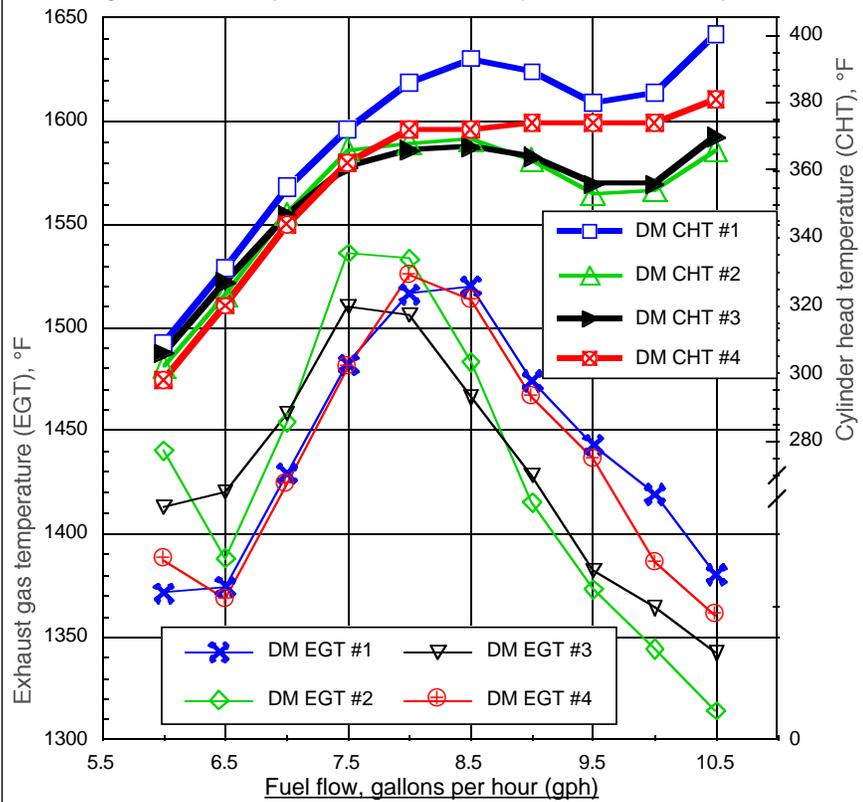
Mooney N6057Q; 15,000' density alt., wide open throttle, 2550 RPM, Vetter DAD records. CHT for 100 °F day. DM = dual Bendix magnetos @ 25° BTDC timing. At 6.0 gph, the rise in EGT due to misfire is greatest for cyl. #2
