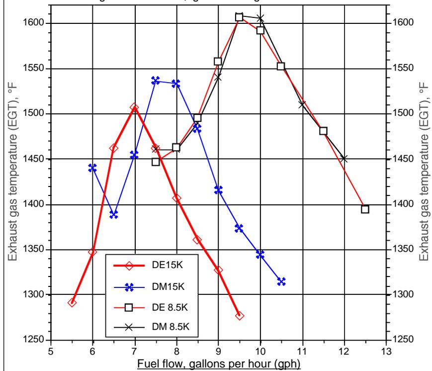
Mooney N6057Q. EGT of cylinder #2 (richest) at 8,500' and 15,000' density altitudes. Wide open throttle, 2550 RPM, wing Barograph #3. Cowl flaps fully opened. DM at 25° BTDC. DE at 30° BTDC @ 8,500' and at 41° BTDC @ 15,000'. Vetter DAD records. DM = dual Bendix 1200 magnetos. DE = dual electronic ignition, Electroair EIS-1.
