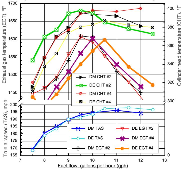
Mooney N6057Q at 8,500' density altitude, wide open throttle, 2550 RPM, richest cylinder #2, leanest cylinder #4. Wing Barograph #3 and Vetter DAD records. DE = dual electronic EIS-1 ignition @ 30° BTDC. DM = dual Bendix 1200 magnetos @ 25° BTDC.
