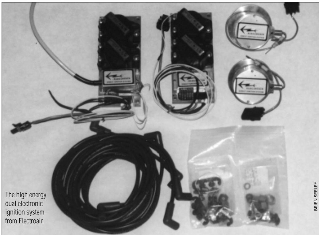
The high energy dual electronic ignition system from Electroair.
