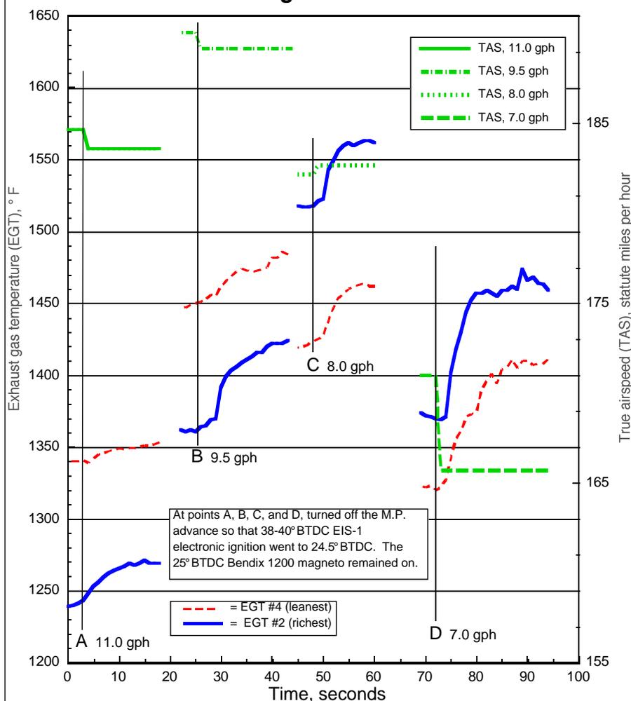
Change in EGT and TAS when ignition timing reduced from ~40° to 24.5° BTDC, 4 different fuel mixtures: Mooney N6057Q, 12/15/01. 12,500' density, w.o.t., 2550 RPM. Bottom spark plugs on Electroair EIS-1. Top spark plugs on Bendix 1200 mag @ 25° BTDC timing.
