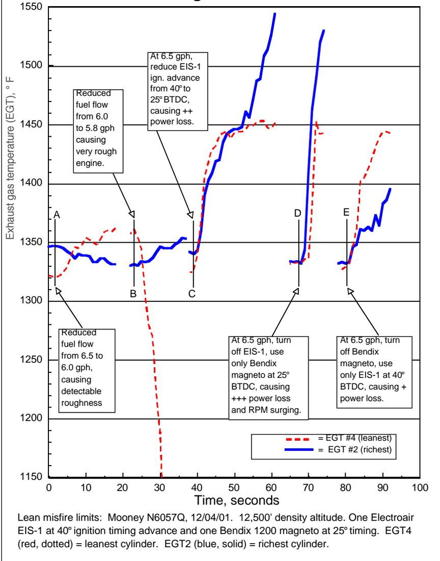
expected, the CHT is hottest and the EGT is coolest with advanced ignition timing. CHT falls dramatically with all configurations as the mixtures are made very lean. Even during the onset of lean misfire, the EGT remains much cooler than peak EGT.
